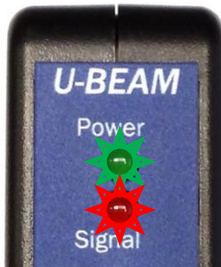
Figure 5. Properly Functioning Controller with U-Beam Sensor Connected and Signal Through
