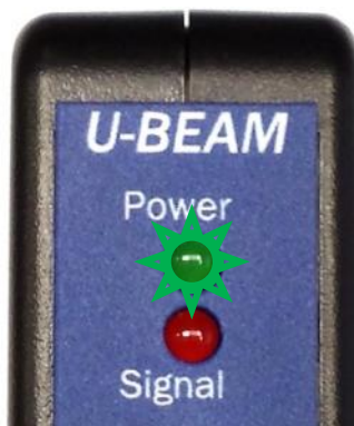
Figure 6. Properly Functioning Controller with U-Beam Sensor Connected and Signal Interruption, Broken Fiber or High Loss
