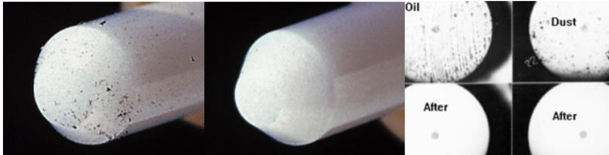
Figure 23. Dirty and Clean Fiber Optic Connector Ferrule and Endface Views.
