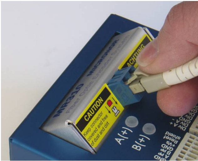
Figure 5. Making Duplex LC Optical Connection to MR320 Controller.
