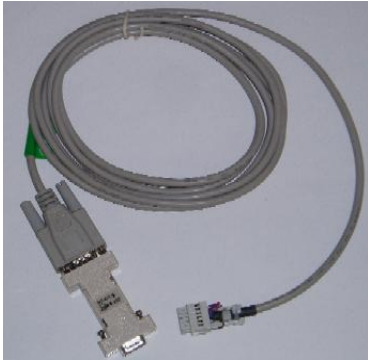
Figure 13. Photograph of MR232-1 RS422/RS485-to-RS232 Adapter Cable.
