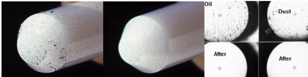
Figure 22. Dirty and Clean Fiber Optic Connector Ferrule and Endface Views.
