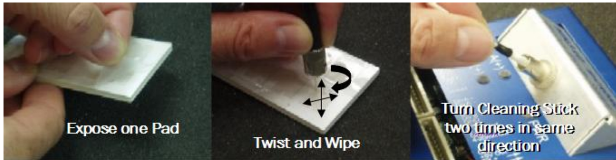
Figure 24. How To Use the MR321 Kit For Cleaning ST Optical Connectors and Interfaces.
