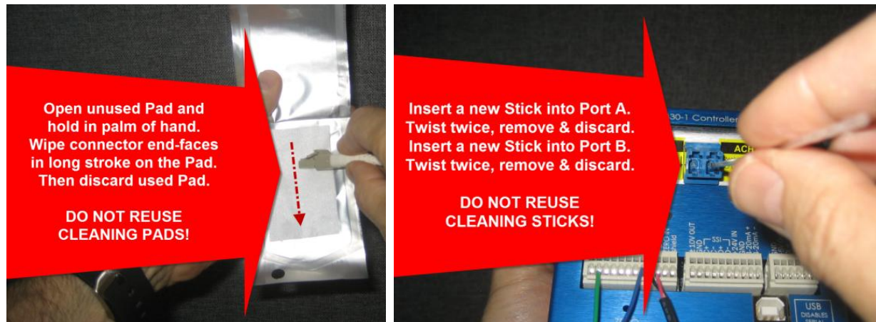
Figure 25. How To Use the MR321C Kit For Cleaning Duplex LC Optical Connectors and Interfaces.
