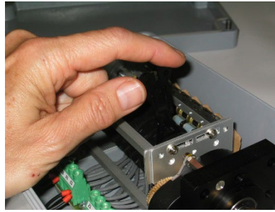
Figure 6. How to Program Cams with the PSN Programming Tool
