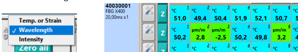
Fig. 7 Dropdown menu for „Measured value“ (left). Sensor fiber containing both strain and temperature FBGs (right).
