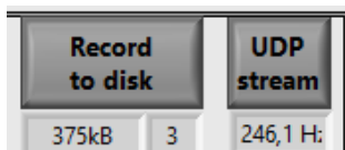
Fig. 18 Activated "Record to disk" button with actual file size ("375kB") and actual file number ("3"). Activated "UDP stream" button with actual streaming frequency ("246.1Hz").
