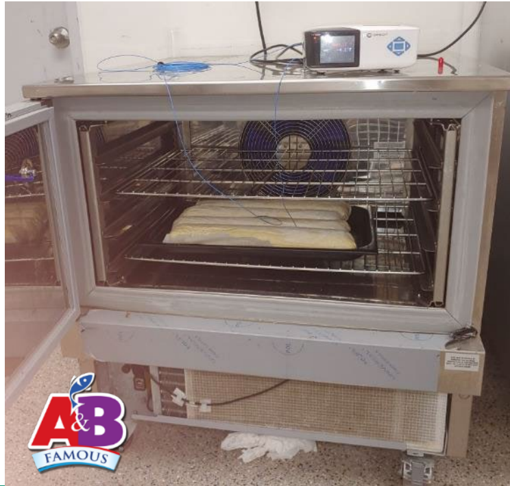
Microwave Food Processing using TS3 GaAs Temperature Probe
