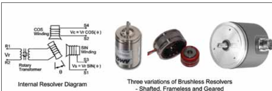
Figure 5—Diagram and examples of resolvers.
