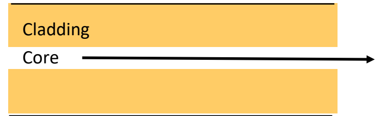
A mode travelling in a singlemode fiber
